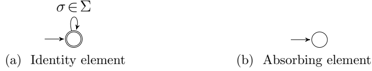
Figure 2: Finite state automata acting as identity element and absorbing element for the automata cross-product operation.
