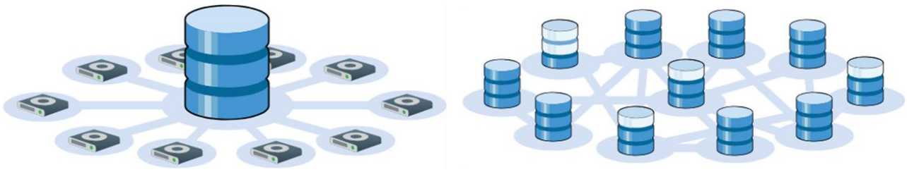
Figure 3: Centralized and distributed architectures. The centralized architecture to the left illustrates a single system retaining the information and offering services to the other nodes in the network. The peer-to-peer network to the right shows a replica of information and services on all nodes. Notice, however, that replicas may not be identical.
